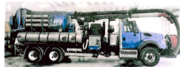
Presents a Proposal Summary of the 2015 Vactor 2112-SE2 Plus Single Engine Hydro Excavation Machine with Positive Displacement Vacuum System Mounted on a Heavy-Duty Truck Chassis
